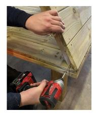
4. Lift the back panel into place ensuring this is flush with the ends of the side panels. Secure in place inside the product using 9 x 80mm screws along the bottom and sides.
